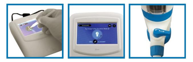
E-burette is commonly used in the titration process to determine the concentration of an unknown solution. Typically, titrant (known solution) is added from a burette to a known volume of analyte (unknown solution) until the reaction is complete. An indicator is used to find the endpoint of the titration.
