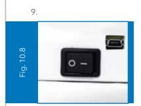
The E-Burette is now ready to be switched on. Press the ON button (of the ON/OFF button) at the back of the control panel to switch on the control panel. (Fig. 10.8)
