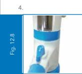
Turn the knob clockwise to set at titration mode and click the tick (✓) mark on the screen of the control panel when ready. (Fig. 12.8)
