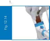
To replace the inspection window, unclip the default inspection window by pressing it from its top and then removing it. (Fig. 12.14)
