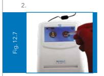
Click on the Titration mode on the home screen. (Fig. 12.7) 3. The screen on the control panel will warn the user to turn the knob to titration mode.
