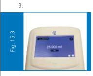
Click the settings icon on the bottom (Fig. 15.1) From the settings menu, choose Calibration. Fill the nominal volume of double distilled de-ionized water by clicking the FILL button on the calibration screen of the operating panel. (Fig. 15.3)
