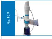
When mounted to a reagent bottle, always carry the instrument as shown and always store it in the upright position. (Fig. 10.9)
