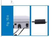
If charging is required, insert the charging pin at the back of the control panel and connect the power cord with the AC adaptor firmly and then plug the two pin power cord to the 220 V power supply. (Fig. 10.6)
