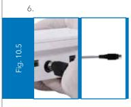
Connect the cable from the instrument housing to the port at the back of the control panel with a firm push, as shown. Check for the cable position. The flat surface of the connector with an arrow mark will face down. (Fig. 10.5)
