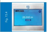
Dispense the filled liquid by clicking on the DISPENSE button on the calibration screen of the control panel. (Fig. 15.4)
