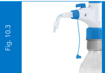
Remove cap from the discharge tube. (Fig. 10.3)
