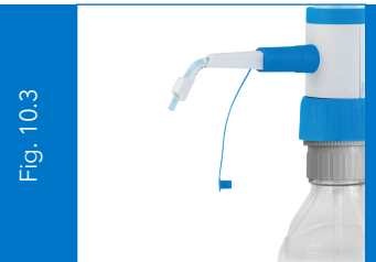
Remove cap from the discharge tube. (Fig. 10.3)
