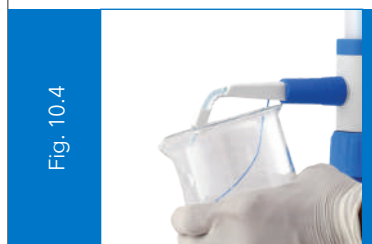
Hold the discharge tube orifice against the inner wall of the appropriate receiving vessel. (Fig. 10.4)
