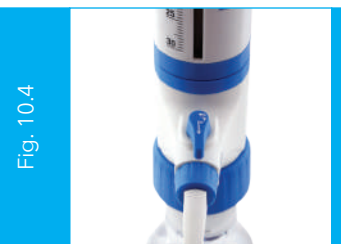
Before using the instrument, turn the valve to 'Dispensing'. (Fig. 10.4)
