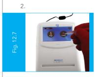
Click on the Titration mode on the home screen. (Fig. 12.7) 3. The screen on the control panel will warn the user to turn the knob to titration mode.
