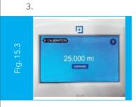
Click the settings icon on the bottom (Fig. 15.1) From the settings menu, choose Calibration. Fill the nominal volume of double distilled de-ionized water by clicking the FILL button on the calibration screen of the operating panel. (Fig. 15.3)
