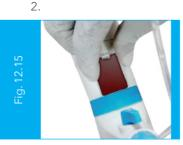
To replace the inspection window, unclip the default inspection window by pressing it from its top and then removing it. (Fig. 12.14) Place the Amber Coloured Window in the slot provided at the bottom of the housing and press it down until you hear a click sound. (Fig. 12.15)
